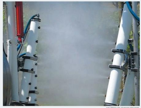
Electrostatic sprayers create a low pressure, low volume concentration.
