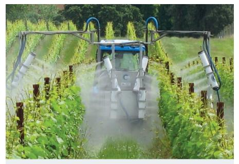
Two-row electrostatic spray booms create a targeted 50-micron fog.
