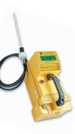
The Eagle meter from RKI with extension tube attached for remote monitoring
