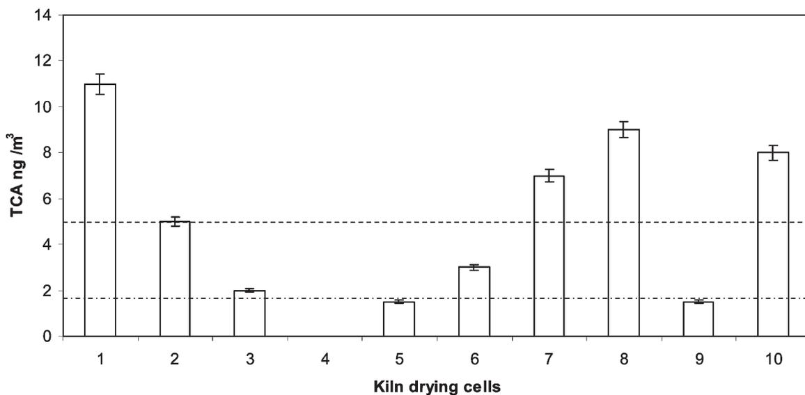
Figure 4. TCA concentration in the kiln oven atmospheres used for oak wood stabilization before barrel making after 24 months of natural seasoning. --- Limit of Detection LOD =  $1.75 \text{ ng/m}^3 \pm 0.75$ . --- Limit of Quantification LOQ =  $5 \text{ ng/m}^3 \pm 2.5$ .
