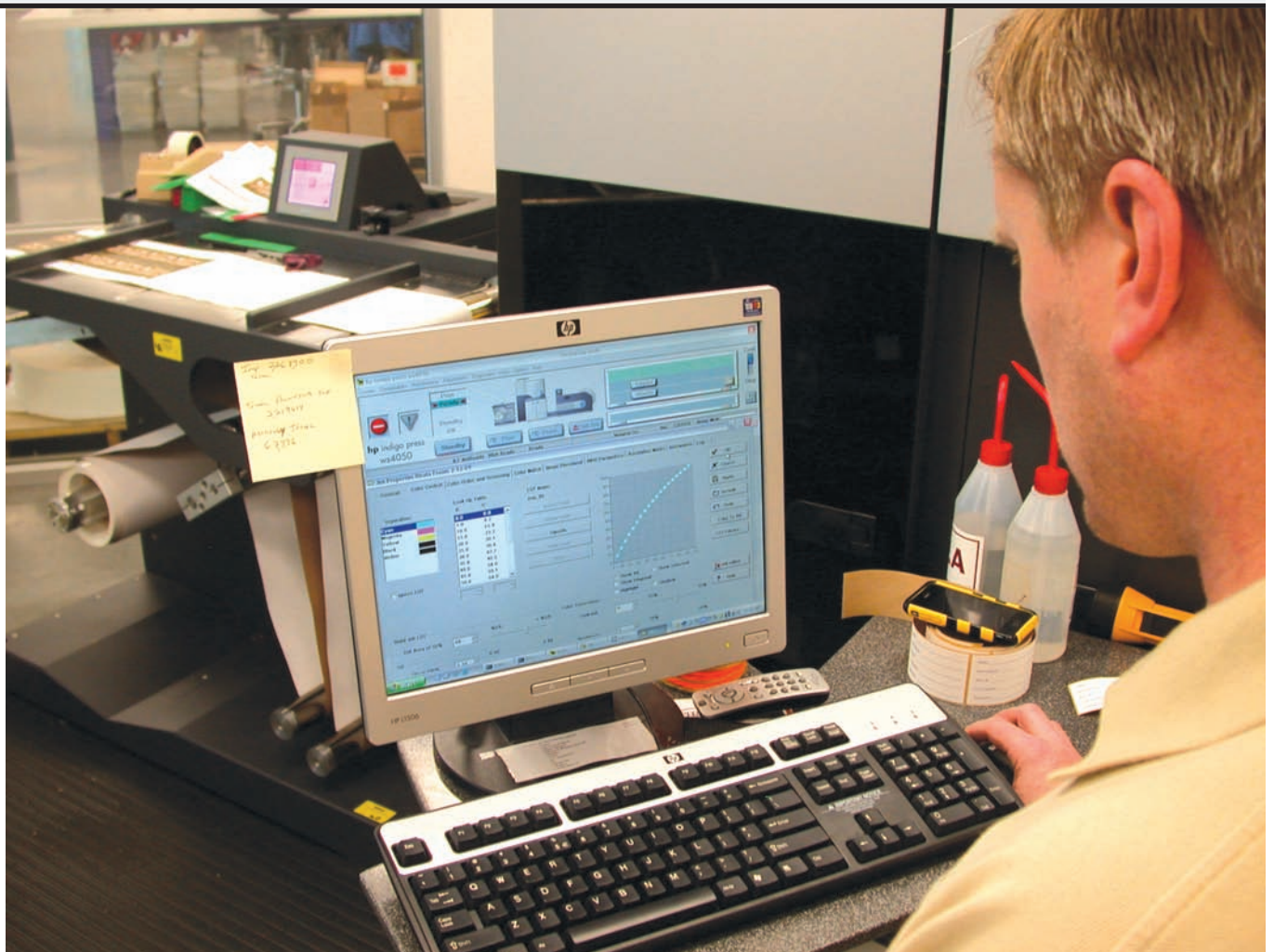
The HP Indigo Press is computer operated so any color changes to final proof takes just minutes.
